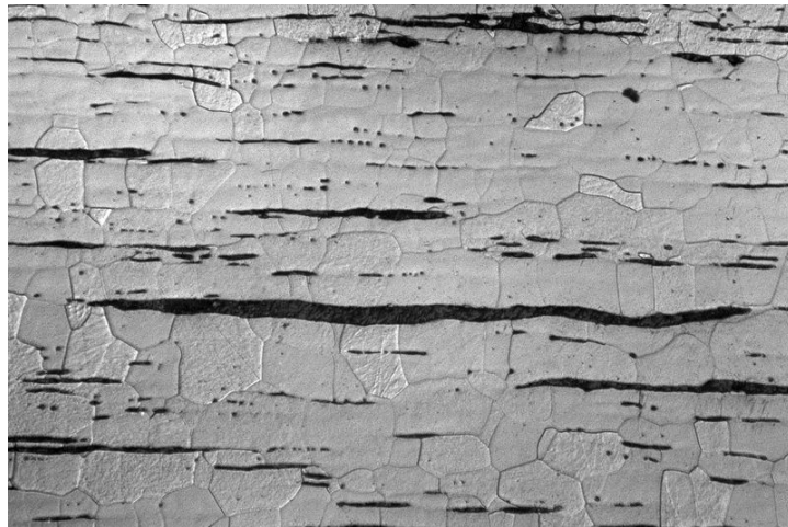
Figure 11.20: Optical Micrograph of wrought iron showing dark slag inclusions in ferrite.
