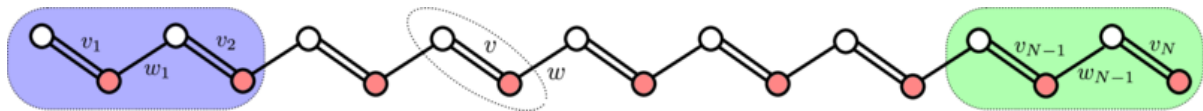
Figure 1.1: Geometry of the SSH model. A 1D chain with two atoms in the unit cell (circled by dashed line). The hopping amplitudes are staggered: w (double line) and v (single line). The long chain consists of the left edge (blue shaded background), the translationally invariant bulk (no background) and the right edge (green shaded background). The hopping amplitudes at the edges are subject to disorder, in the bulk, however, are fixed. .
